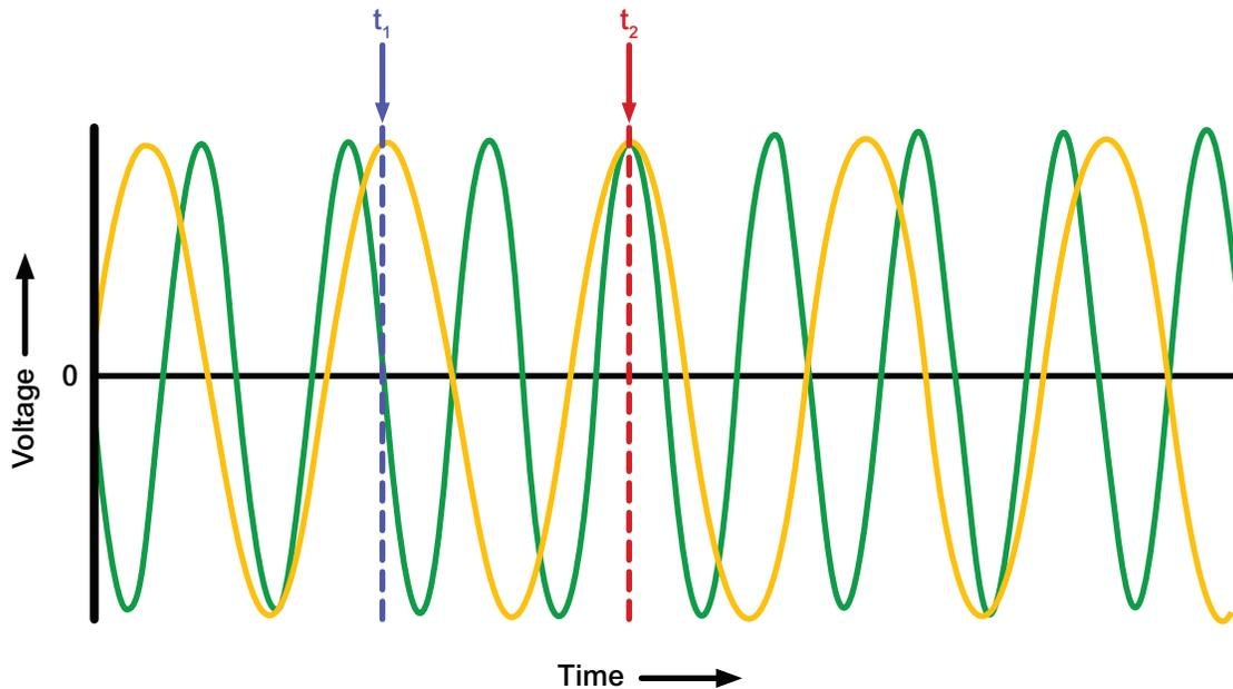
Figure 1: In-rush current at  $t_1$ , where the phase angle difference is  $\sim 90$  degrees, would be much greater than at  $t_2$ , where the difference approaches zero degrees. In normal applications, the frequencies would vary less widely than shown.
