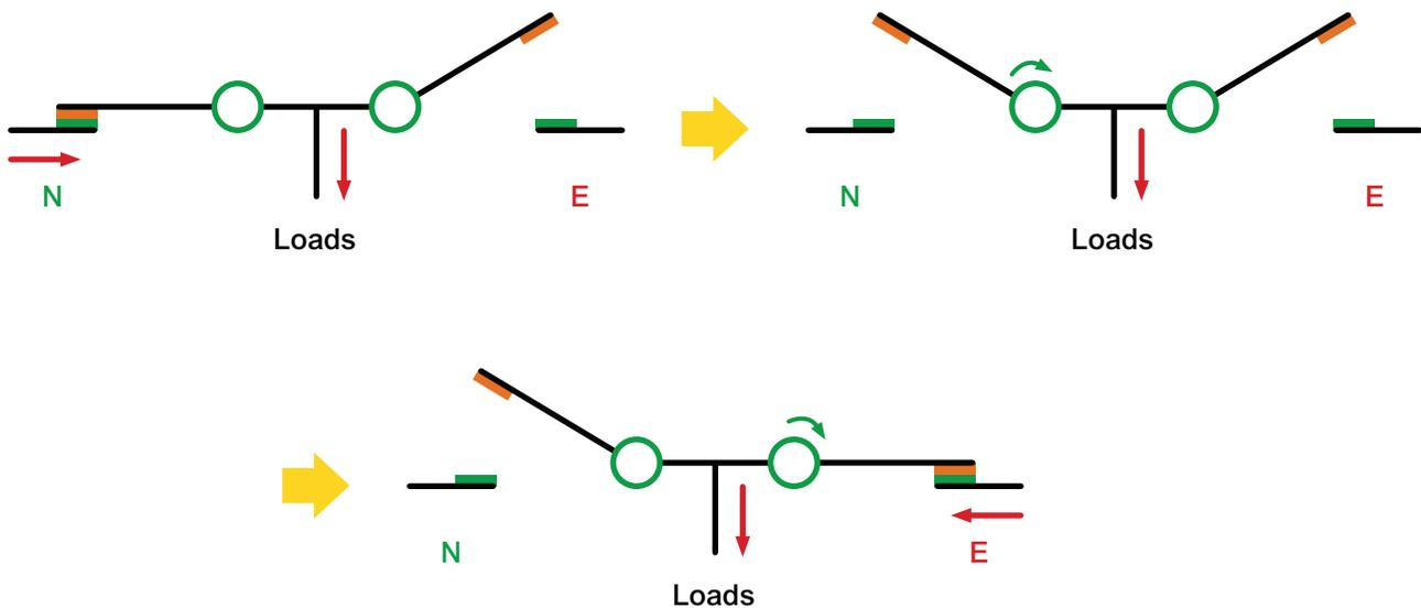
**Figure 3: A delayed transition sequence, where the transfer mechanism contacts disconnect from the Normal source, hold a center-off position, then connect to the Emergency source.**
