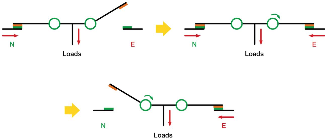
Figure 4: A closed transition sequence where the Normal and Emergency sources are momentarily paralleled.
