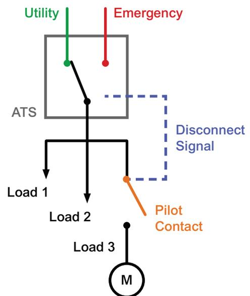
Figure 2: A motor load disconnect circuit solution
