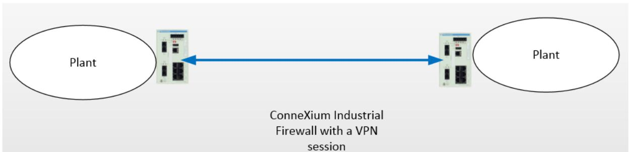
**Figure 28: VPN Tunnel for Plant to Plant Secure Communication**
