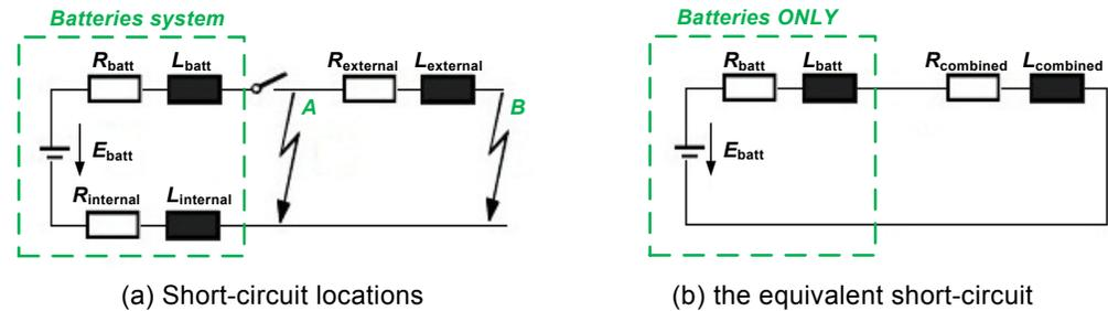
The inductances ( $L_{batt}$  and  $L_{combined}$ ) shown in **Figure 3b** limit the short-circuit current initial rate of rise to a peak value ( $I_p$ ) at time ( $t_p$ ), but not the short-circuit current ( $I_{sc}$ ) which trips the protection devices shown in **Figure 4**. The short-circuit current, which helps to set the trip current of the protection devices, can be calculated using the following formula:
