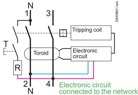
In the case of VDT technology ("Voltage Dependent Technology"), the toroid only provides information about the leakage current. The power required for tripping is supplied by the electrical network.
