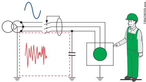
As RCDs are designed to detect very low currents (e.g.: 30 mA), interference due to the network or its environment can, in certain cases, result in RCD tripping.
