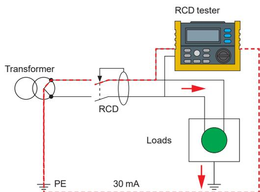
→ Earth leakage current
