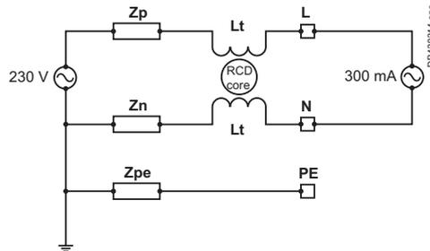
In this case measurement current pass through the 2 RCD windings in opposite polarity and the total Self  $L = L_t - L_t \sim 0$ . (magnetic leakage is negligible).
