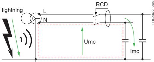
Fig. 1: lightning current discharge to earth
