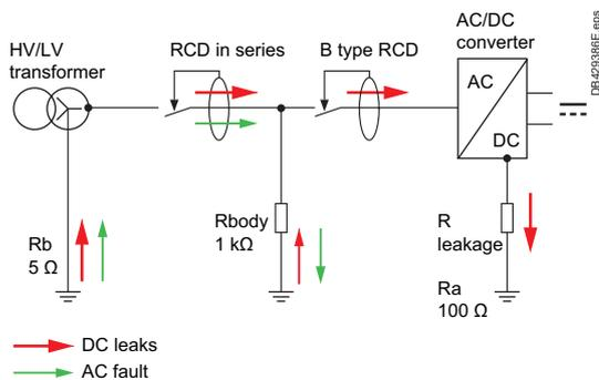
The DC leakage current generated by the DC voltage source and produced by the AC/DC converter (DC bus) only flows through the RCDs connected in parallel in the event of an insulation fault in a parallel load or in the event of contact with the parallel outgoer.
