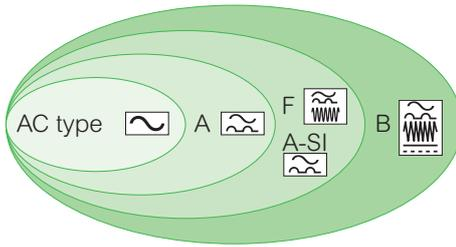
The increase in use of electronic loads can result in earth leakage current with different waveform characteristics. This situation must be carefully analyzed as it affects the performance of RCD. That is why the IEC series of standards has defined four types of RCD.
