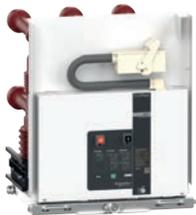
The EvoPact HVX fixed type is equipped with drilled and threaded copper connection terminals at the top and bottom
