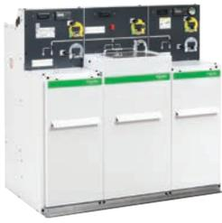
The RM6 is a compact and very reliable Gas Insulated ring main unit combining all MV functional Units to enable the connection, supply and protection of transformers or feeders on an open ring or radial network. Together with Easergy T300 RTUs, it is smarter and meets the needs of utilities, infrastructure, buildings & industries.
