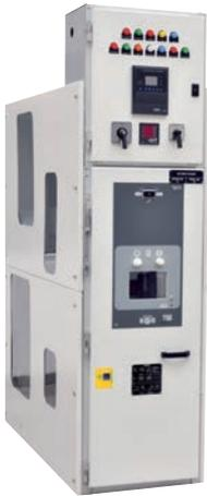
A high performance and a high-quality Air Insulated Switchgear with a floor rolling Vacuum Circuit Breaker up to 17.5 kV, 31.5 kA and 2500 A.
