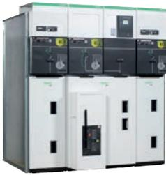
A high performance and a high-quality Air Insulated Switchgear with a floor rolling Vacuum Circuit Breaker up to 17.5 kV, 31.5 kA and 2500 A.
