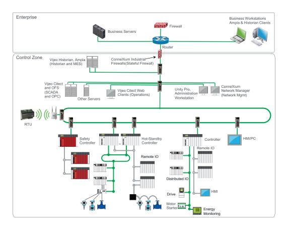
ICS components are deployed throughout the network, including controllers, safety systems, drives, and HMIs. The sample network is a generic industrial control system that could be used in a variety of industrial segments.
