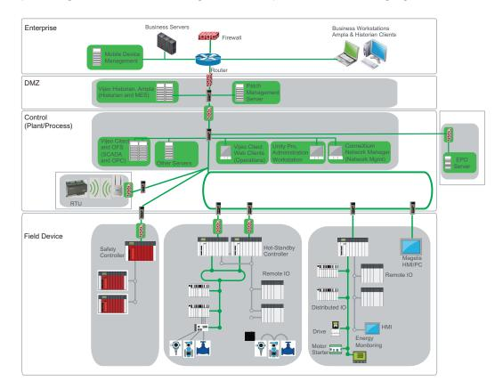
In this example, the control zone from the sample network has been broken into seven smaller zones highlighted in grey. New elements are highlighted in green. The zones are:
