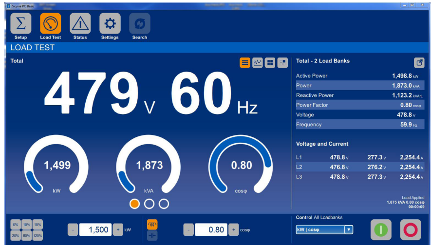
This is a screen shot of software showing power factor rating. (Photo courtesy of ASCO Power Technologies.)
