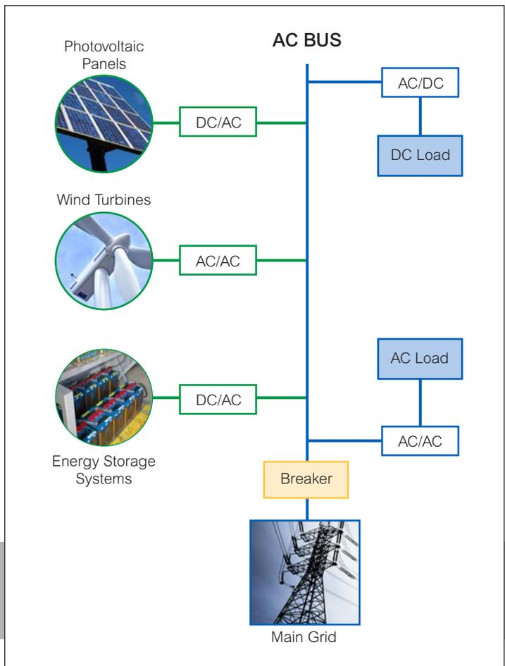
FIGURE 3: An example of typical AC Energy Storage System.
