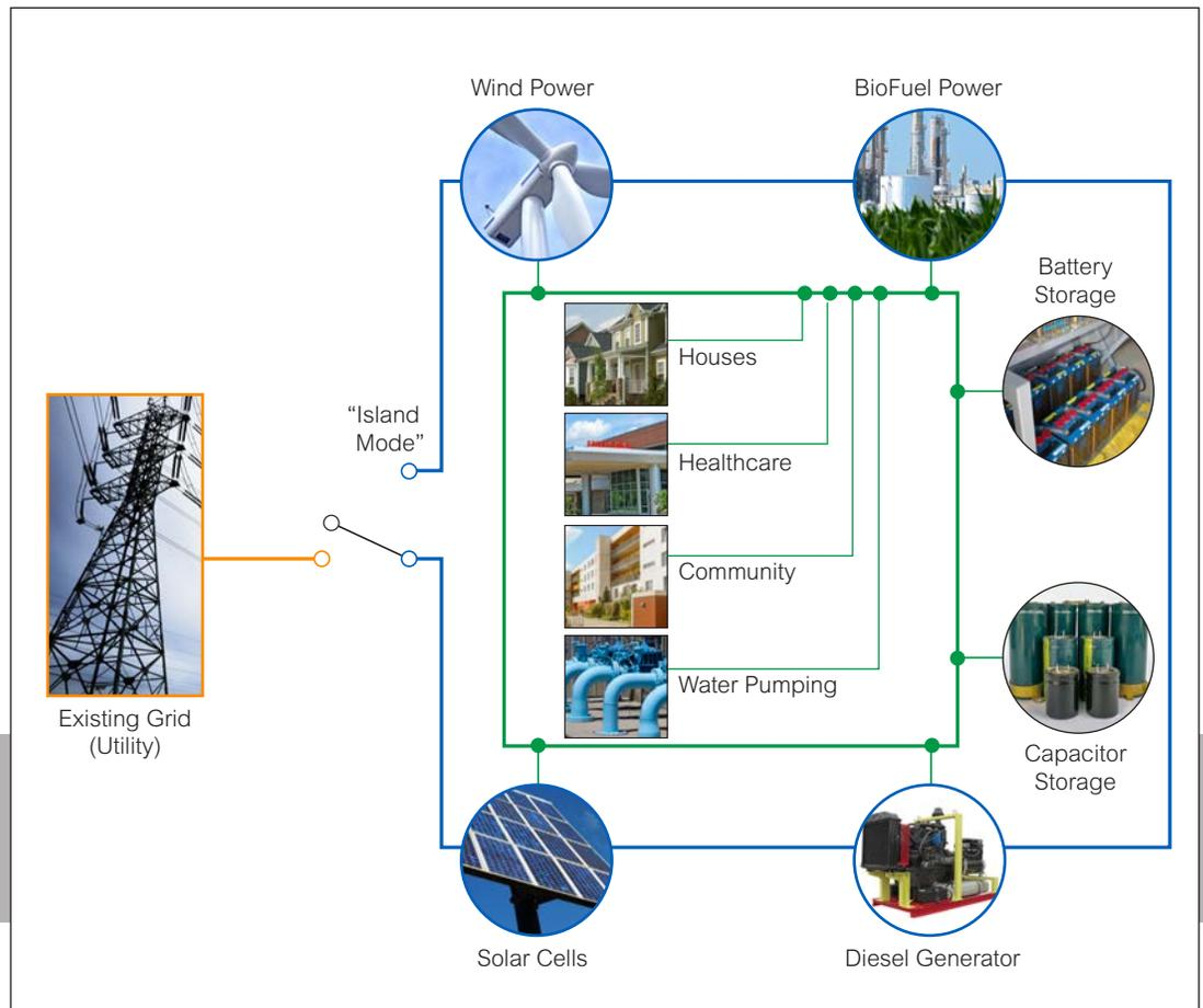
FIGURE 1: Example of microgrid configuration.
