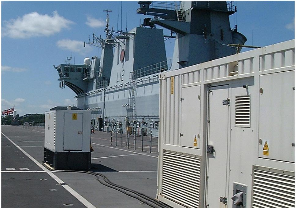
A containerized load bank solution testing a diesel gen-set on a naval vessel.
