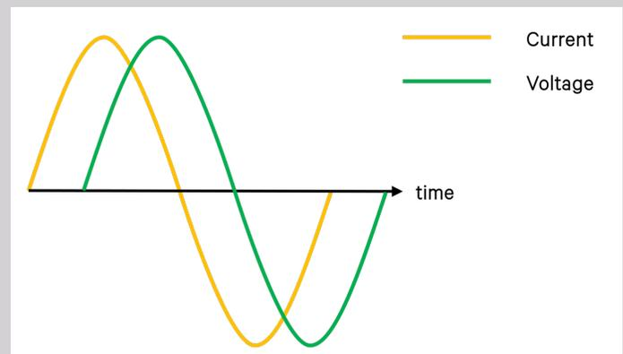
Figure 2: Negative Reactive Power. Voltage trails current.
