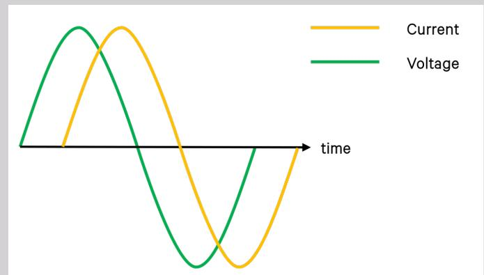
Figure 1: Positive Reactive Power. Voltage leads current.
