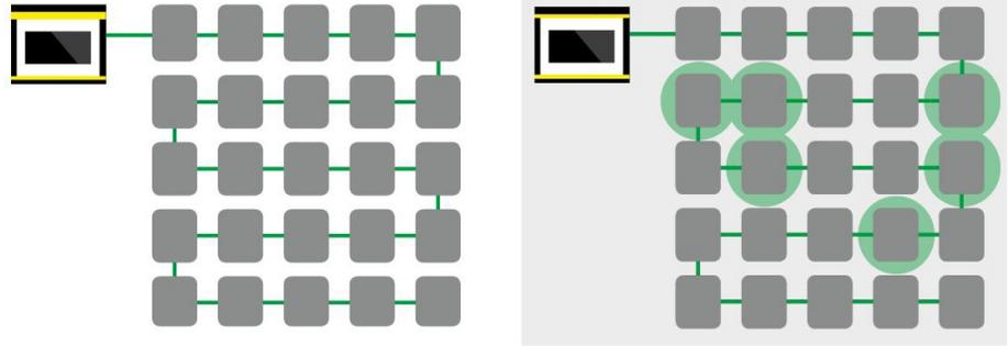
**Figure 2. Left: A single remote control can connect many load banks together. Right: Load can be applied proportionally to all or specific load banks in a network.**
