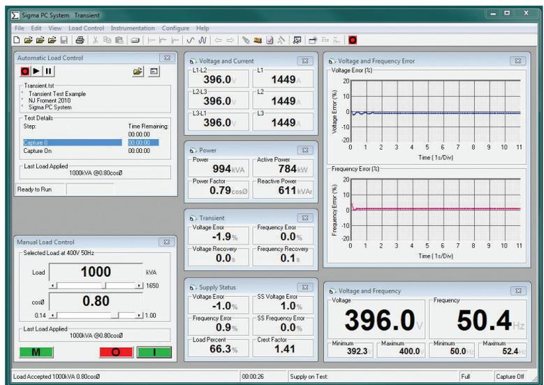
Figure 1. Graphical displays are particularly useful in transient response load tests.
