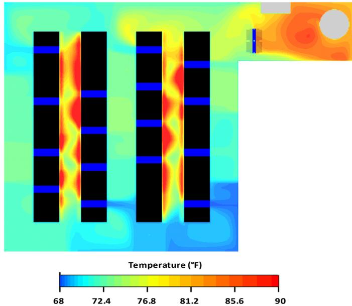
**Figure 6b** illustrates that adding two row-based coolers in the alcove area helps to cool the alcove to within the defined allowable temperatures, although, due to the geometry of the room, the temperature is still slightly warmer than the row-based-cooled area.
