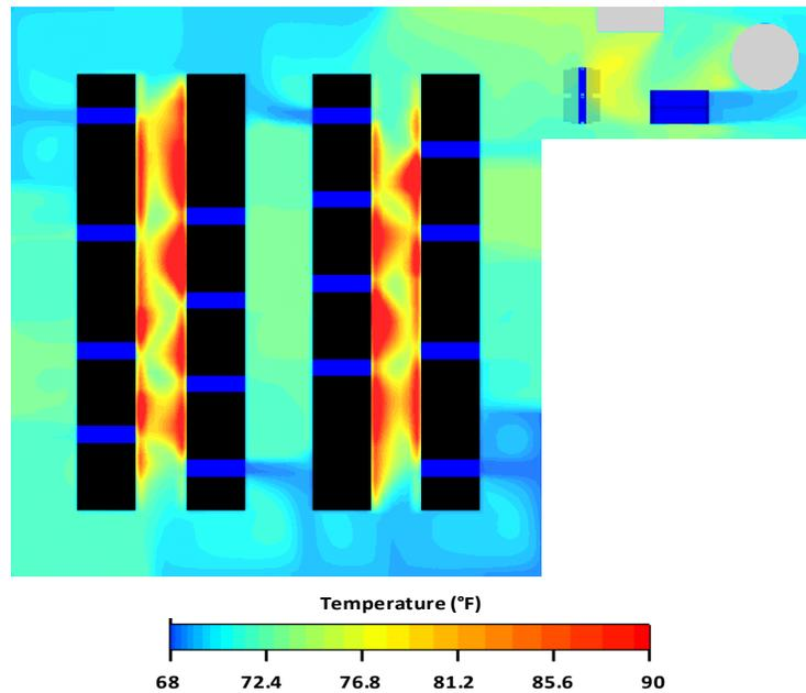
**Figure 6c** shows the scenario where no alcove exists. When a data center has standard room geometry like this example, additional cooling is often unnecessary. The row-based coolers in the 4 rows of racks are sufficient to cool not only the loads they were designed to handle, but also to pick up the additional heat load of the ancillary loads. Temperatures in the ancillary area, although warmer than the temperatures in the rows, are still below the design threshold.
