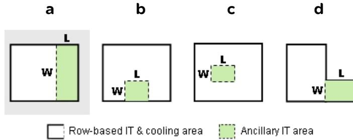
For fixed densities, the temperature in the ancillary area increases slowly with an increase in ancillary area or a decrease in row-based area since these scenarios lead to a greater fraction of un-cooled ancillary area in the data center. The temperature in the row-based area is less affected by the room geometry as the additional heat load is distributed fairly uniformly across the data center as discussed above.
