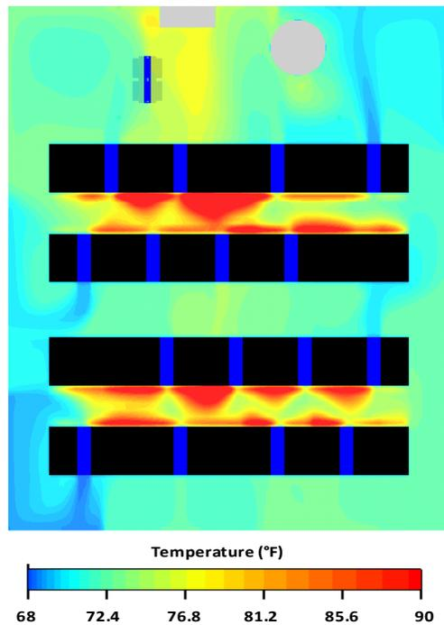
Consistent with the CFD analysis shown for the three scenarios, the InRow Ancillary IT Equipment Cooling Calculator TradeOff Tool predicts that the layout with the alcove requires additional cooling while the layout without the alcove does not.
