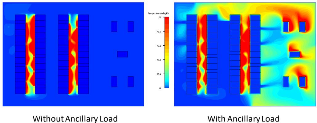
Based on the CFD models and heat balance equations, a model was developed that identifies the parameters affecting the temperature rise in both the row-based and ancillary areas, in order to determine the practical limits of using row coolers to cool ancillary devices. The parameters that affect whether this approach will be effective fall under three categories:
