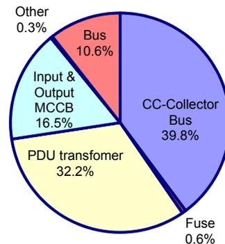
Failures in the PDU transformer and catastrophic failure of the collector bus (the point of parallel connection between power modules and the bypass switch) account for 72% of all expected failures. The input and output molded case circuit breakers account for nearly 17%, despite component failure rates of  $1.2 \times 10^{-7}$  per hour, equivalent to a MTTF of 8.3 million hours.
