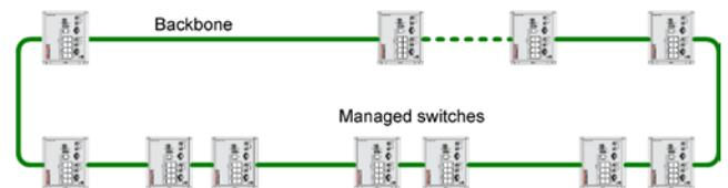
The only disadvantage of ring topology is the absence of an international standard. This results in different implementations of ring recovery depending on the switches manufacturer. Therefore, all the switches in the ring must come from the same manufacturer.
