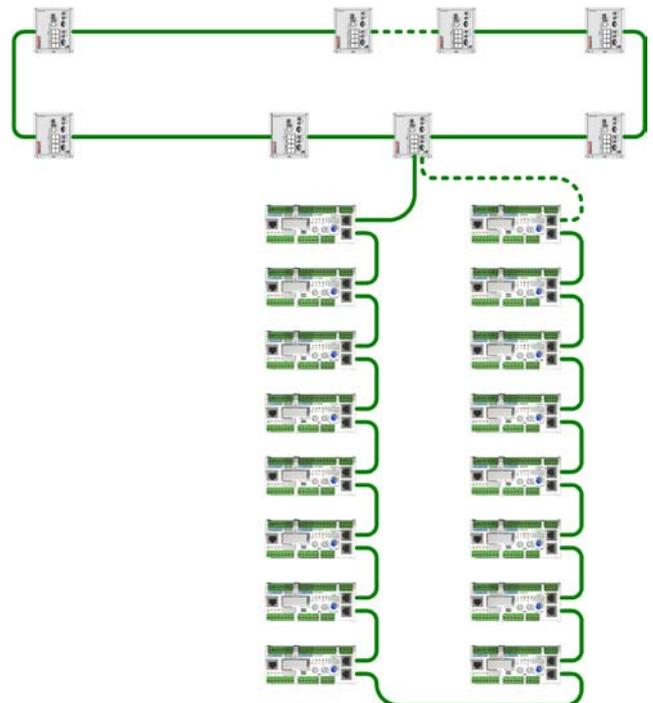
We can solve this problem by looping the daisy chain to a different switch. We call this topology a "Daisy Chain Loop with 2 ring switches".
