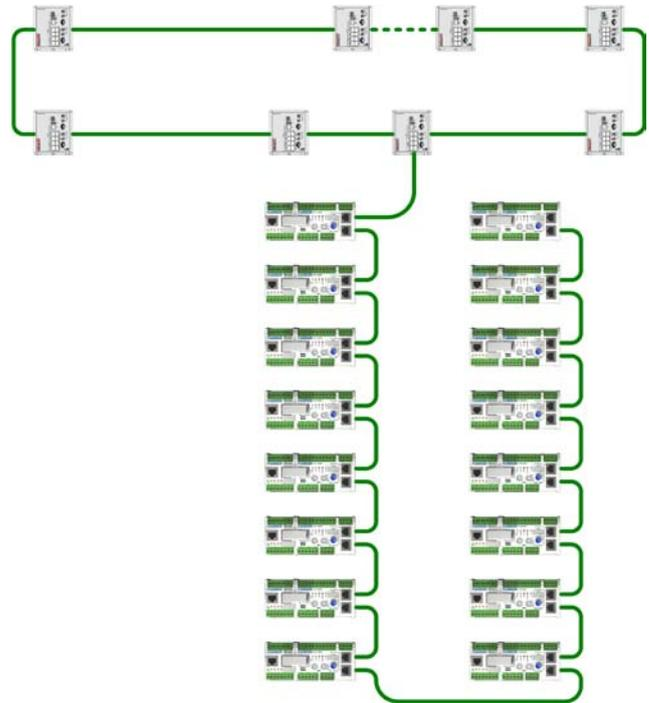
Therefore, a daisy chain must always be looped. The loop creates a *de facto* ring with the same failover characteristics as the backbone ring. This is called a daisy chain loop (hereafter "DCL").
