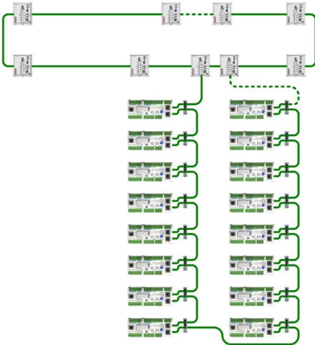
In this way, we obtain a self-healing DCL. Self-healing is done automatically and in complete transparency for the operator.
