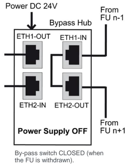
The opening and the closing of the by-pass switch should be automatically executed when the position of the FU changes.
