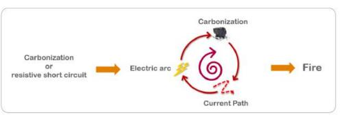
In any building environment where cables are used to transport and distribute electricity, two types of arc fault-related events could occur and lead to a fire:
