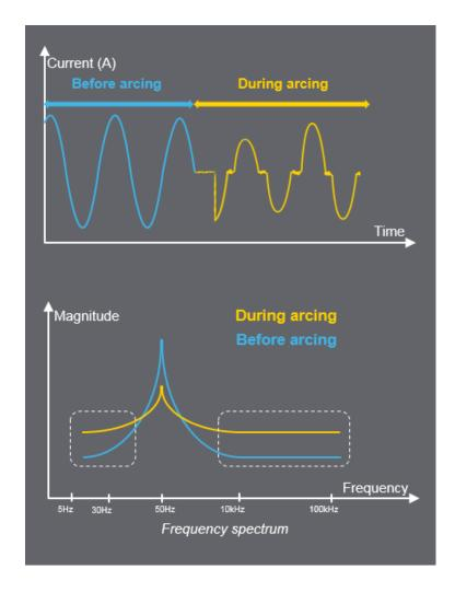
AFDDs cross reference information involving several different electrical parameters in order to ensure that arc fault detection devices are only activated by the appearance of dangerous arcs.
