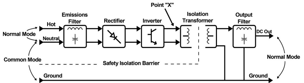
One interesting feature to note in the diagram is that there is actually no physical wire connection between the noisy power lines and the power supply output. In fact, international safety agency requirements stipulate that there must be a minimum of 1/2 cm of physical spacing between input and output. Power is transferred using the magnetic field coupling of an isolation transformer.
