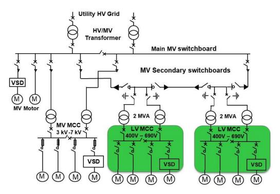
Figure 2 shows a typical MCC consisting of a main busbar that distributes power horizontally between various switchboard columns, and distribution busbars supplying motor starters.
