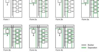
To answer the installation needs, the degree of operator safety and the service continuity required, Table 7 shows the different options related to mechanical parameters such as the form of separation and the type of electrical connections.
