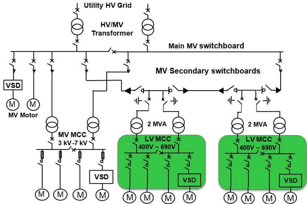
Figure 2 shows a typical MCC consisting of a main busbar that distributes power horizontally between various switchboard columns, and distribution busbars supplying motor starters.
