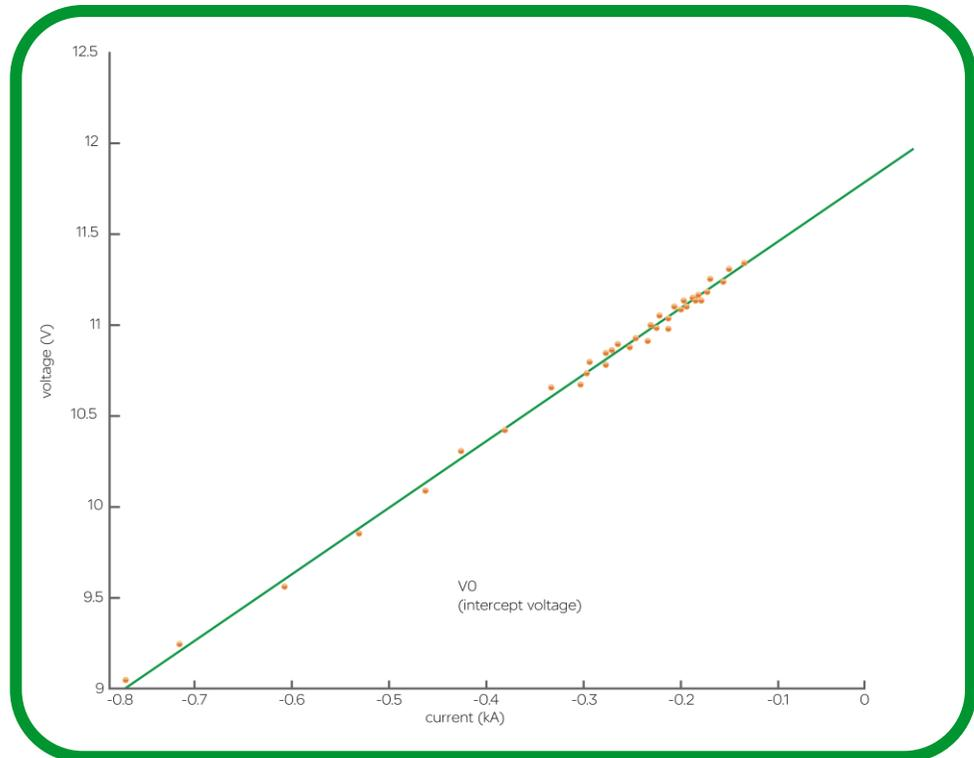
Using battery cranking voltage to gauge the health of a battery also has its advantages. It is an accurate and efficient depiction of the battery dynamics that occur within the cells, during engine cranking as well as startups. Such an approach does not require the addition of costly sensors. These readings can also be compared with previous tests to compare the degradation of the battery(ies).
