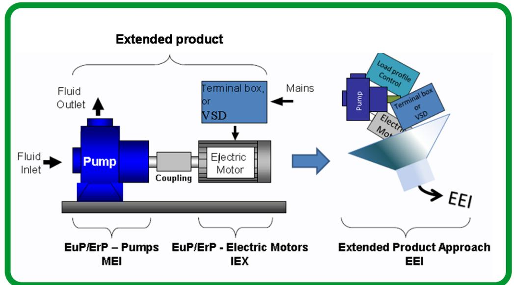
The marketplace is now shifting in order to accommodate these more stringent efficiency regulations. The concept of the "Smart Pumping" which is also termed as “intelligent” pumping system combines higher efficiencies with sensor and software driven ability to regulate and control flow or pressure. This approach results in energy savings, increased equipment lifetime, and maintenance cost reductions.
