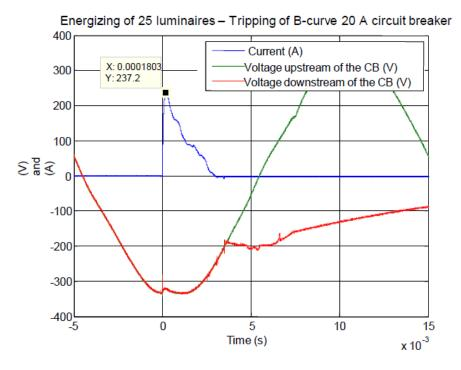
In order to address this situation, an appropriate choice of the circuit breaker device must be made during the design phase (see Figures 11a, 11b and 11c). The peak value of the current at switching on depends on the energizing time, the number of luminaires forming the lighting circuit, and the short-circuit power and architecture of the network.
