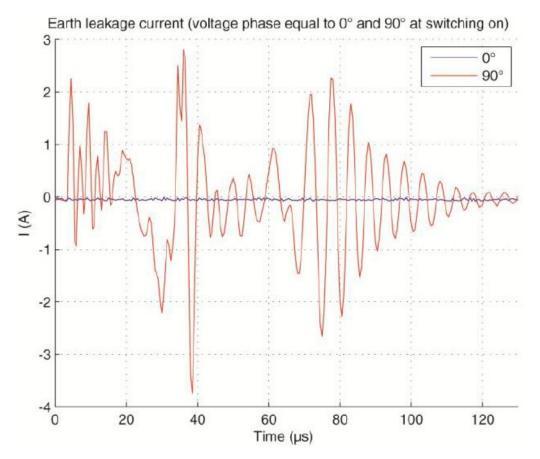
The permanent earth leakage current at 50 Hz is generally less than 1 mA for a luminaire. Given that lighting circuits are protected by earth leakage protection devices of 300 mA rating, many luminaires can be installed downstream of a protective device. For a frequency of 100 kHz, the current is not detected by the earth leakage protection devices.
