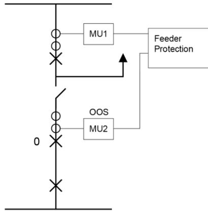
Operation with a missing CT is not unique to breaker and a half substations, similar situations can occur with multiple winding transformers (dual secondary or tertiary windings). In these cases, the winding remains energised, however, it is unloaded by isolating the winding effectively taking it out of service.
