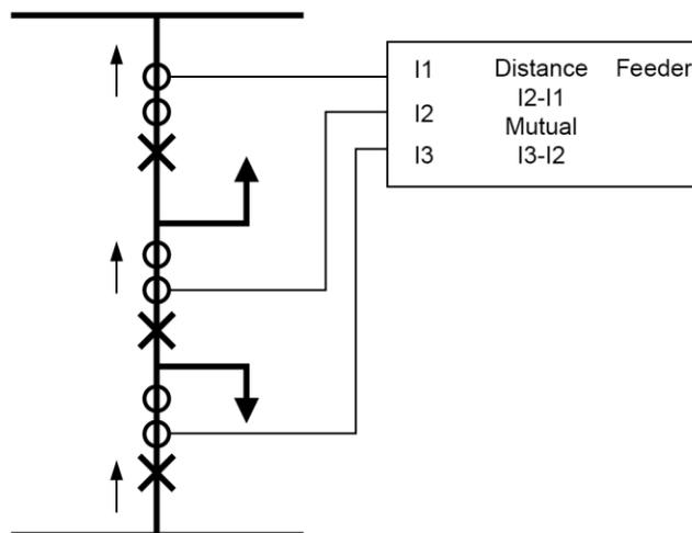
Also, there may be cases where CT1 for example has its polarity reversed. In this case the protection needs  $CT2+CT1$ .
