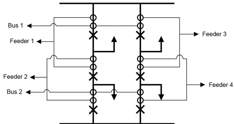
Other applications such as feeder differential and transformer differential require the diameter CTs segregated to avoid operation on diameter through faults. Even in these applications the CTs are often later paralleled and summated, for example, to provide mutual coupling currents for another feeder. This paralleling or addition of currents is traditionally done by simply connecting the CT wiring before or after the protection inputs as required.
