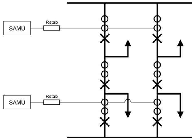
Such an approach could be applied to mutual currents and VSS schemes and may well be practical for retrofit applications. However, for a new installation it offers few benefits. The CTs cannot be used for other protection and therefore require additional cores. New technologies such as NCITs cannot be paralleled or switched and therefore such an approach cannot be used.
