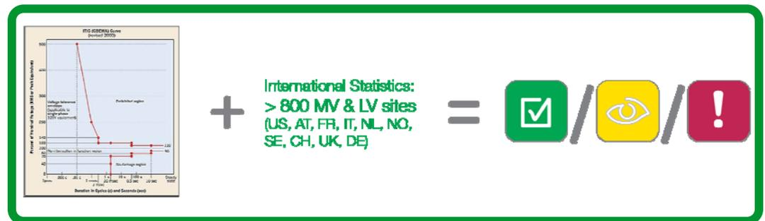
To classify each event, we use the CBEMA-ITIC power acceptability curve (**Figure 1**) or equivalent, on which we plot the magnitude and duration of each individual power quality event to catalog it within two categories:
