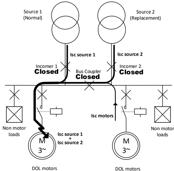
Although compliance with this constraint is not mentioned or required in IEC standards, it is nevertheless clearly stated in Sections 110.9 and 705.16 of the National Electric Code [1]. Therefore, many end-users operating critical processes still specify switchboard short-circuit withstand accordingly. Such a provision generally significantly increases the cost and size of the switchboards. The cost-effectiveness of the entire electrical system can also be affected as follows:
