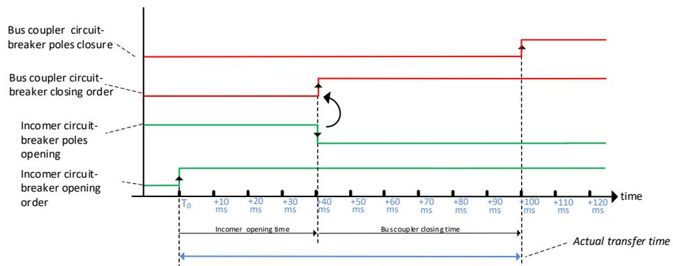
The main drawback of a sequential fast transfer is that the total transfer time cannot be shorter than the sum of the latency values for each circuit breaker. This is typically 100ms for standard low-voltage circuit breakers, and slightly longer for medium-voltage vacuum circuit breakers. This transfer time can exceed requirements, especially in low-voltage applications, to ensure a satisfactory transfer performance according to the requirements of the ANSI C50.41-2012 standard.
