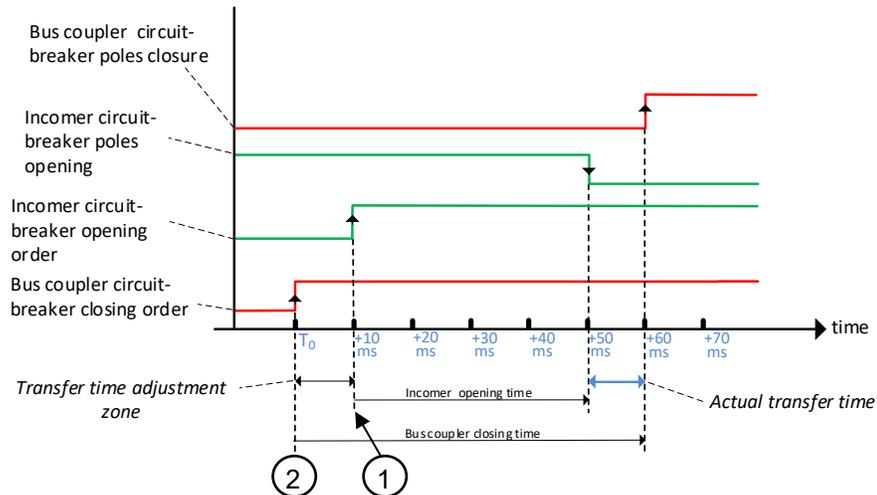
As explained above, a simultaneous fast transfer offers excellent conditions for a source replacement, ensuring a smooth load transfer from one source to another because the bus voltage decay and phase shift can both be extremely low at the instant of the reconnection. The next section explains how motor characteristics and load inertia are important from this standpoint. This method generally exceeds the performance required by the ANSI C50.41-2012 standard.
