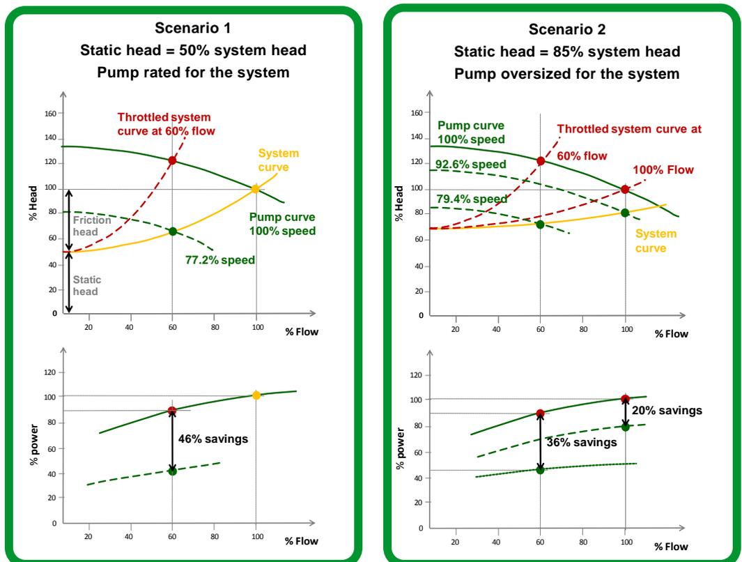
The example in **Figure 2** on page 3 compares two installations (one with a variable speed drive one with a fixed drive throttled system) in which static heads (height difference between the source and the end use) are different.
