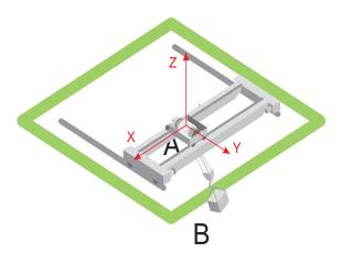
In order to ensure that the operator can deposit the load accurately, the pendulum swaying must be as weak as possible.
