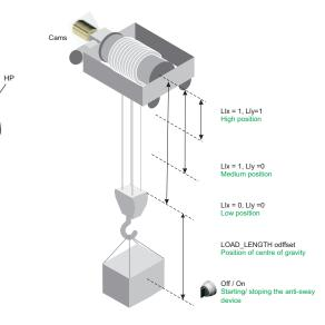
All that will be necessary will be to connect the switches to the corresponding inputs of the function module and to configure the position of the load's centre of gravity.
