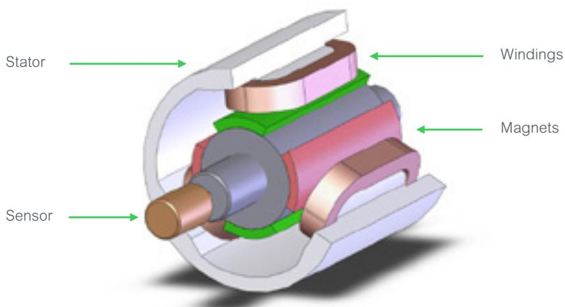
The stator has an embedded three-phase winding. The rotor, made of both north pole and south pole magnetic materials, are represented in green and red. The synchronous motor is connected to an electronic drive that ensures the servo control. This is why it's represented as a sensor connected to the shaft.
