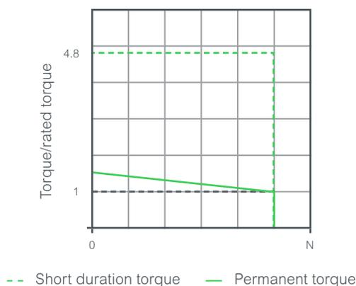
Its nominal torque is 5.2 Nm at 3,000 rpm, which produces 1.6 kW.
