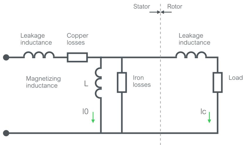
If we neglected the windings' resistance, we saw that the voltage applied to the magnetizing coil noted L created a current named I<sub>0</sub>.
