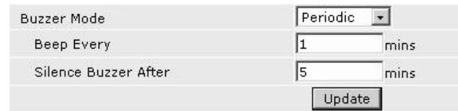
Figure 8: Audible Alarm (buzzer) ON - OFF Times
