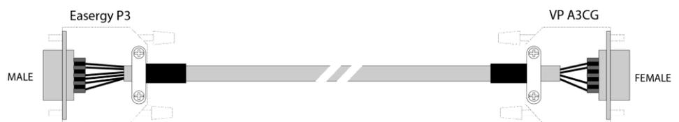
Figure 3.. Profibus cable REL52824 (VX072) for Easergy P3 Advanced
