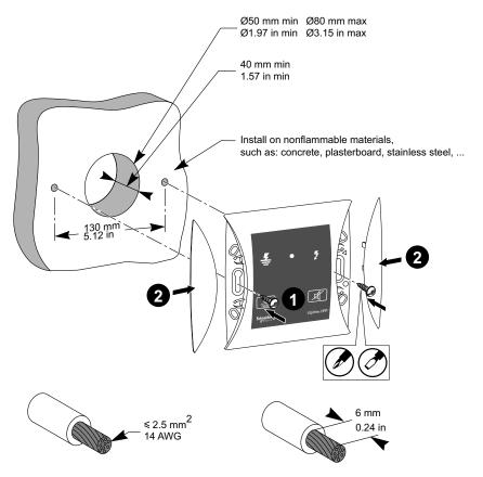
The HRP is connected to the insulation alarm relay terminal block. See wiring diagram from the device to the HRP (Wiring diagram, page 19). The connector details of HRP is illustrated in the following figure:
