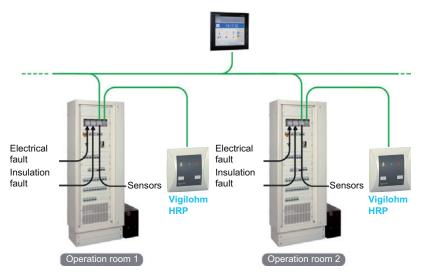
The HRP connection principle is illustrated in the following figure:
