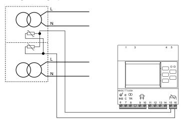
If the transformer has three columns, wire the third temperature sensor in parallel with the other two sensors.
