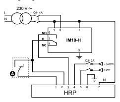
Wiring diagram from IM15H / IM20-H to HRP:
