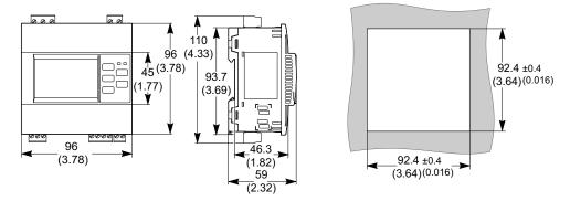
Observe the correct distances between devices for flush-mounting as per the following figure:
