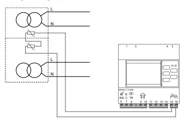
If the transformer has three columns, wire the third temperature sensor in series with the other two sensors.
