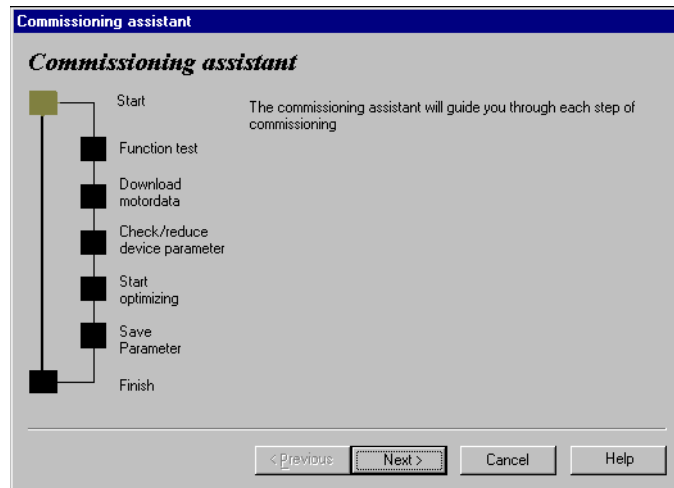
Figure 5.5 Commissioning with the wizards
