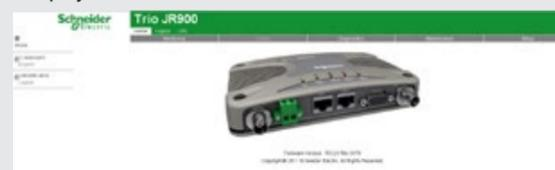
It may be necessary to disable a web proxy (if in use) or disable/modify a local firewall to help ensure the security rules allow access to the J Series IP address.
