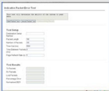
When the test is complete, a message stating "Packet error test completed" is shown and the test results summarised in the "Test Results" section.
