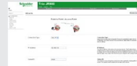
The Subnet ID should be a descriptive text name for the radio link and identical in both Access Point and Remote radios, for correct operation. The configuration cannot be saved with the factory default Subnet ID. Choose a unique ID and record it for future use. Up to 20 printable characters can be used.
