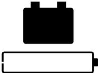
The Back-UPS is operating on battery power and the battery power is getting low. Shut down all connected equipment to avoid losing an unsaved data. When possible, connect the Back-UPS to AC power to recharge the battery.
