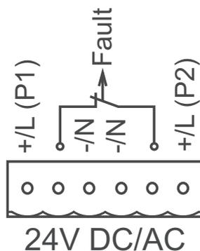
Figure 2: Pin assignment of the 6-pin terminal block
