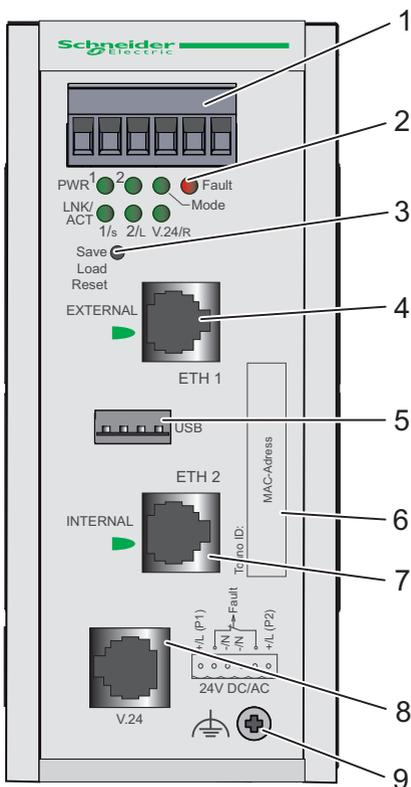
Figure 1: Overview of interfaces and display and operating elements in the TCSEFEA
