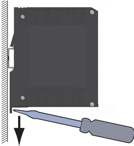
Figure 4: Removing the device from the DIN rail
