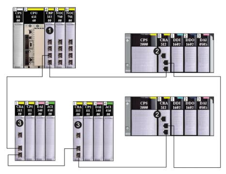
1 local rack with a 140CRP31200 remote I/O head module
