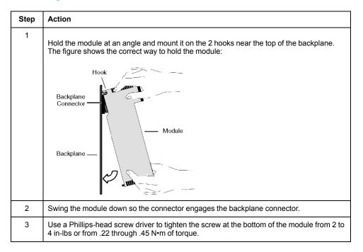
**NOTE:** The figure above shows a **Quantum** module being mounted from top to bottom. Modicon X80 modules mount from bottom to top.
