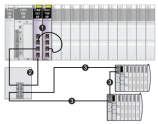
**1** local rack, including a 140 NOC 780 00 distributed I/O head module that is interlinked with a 140CRP31200 remote I/O head module
