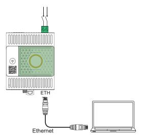
Proceed as follows to connect a PC to a Panel Server through Ethernet:
