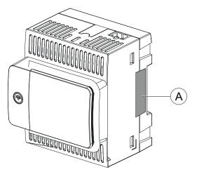
Before installing, operating, servicing, or maintaining the EcoStruxure Panel Server, check the tamper-indicating label integrity.
