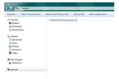
4. Wait until the EcoStruxure Panel Server icon displays in the list of devices in the network. It may take up to 2 minutes after the Panel Server is powered on.
