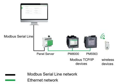
The Modbus-SL reverse mode can be set and monitored on the Panel Server webpages at **Settings > Modbus Devices**. In **Modbus configuration** change the **Modbus mode** from **Client** to **Server**.
