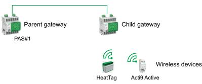
**NOTE:** Panel Server Universal and Advanced allow you to display data from wireless devices connected to a child gateway. The parent Panel Server gateway monitors the Modbus TCP/IP communication status of the child gateway and its downstream wireless devices, and reports an alarm when the child gateway disconnects.
