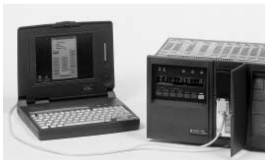
ACE 900 adapter to be connected to the pocket terminal socket.
