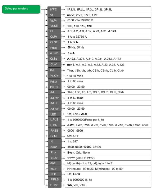
**NOTE:** The setup parameters CoM, Id, bAud, Prty, YEAr,. dAtE, and hour are applicable for the commercial references METSEEM6400NGRSCL1, METSEEM6400NGRSCL5, and METSEEM6400NGRSCL2. The setup parameters PoP, P.PLS, and P.PAr are available for the commercial references.METSEEM6400NGPOCL1, and METSEEM6400NGPOCL5.
