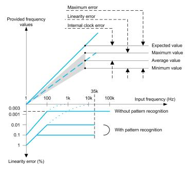
For each input frequency, the module provides frequency values close to the expected value (theoretical value).
