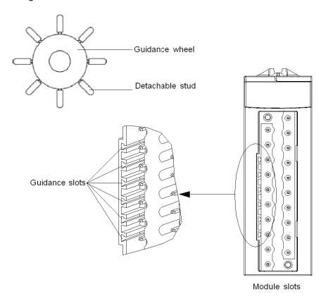
The following example depicts a coding configuration that allows a terminal block to fit together with a module:
