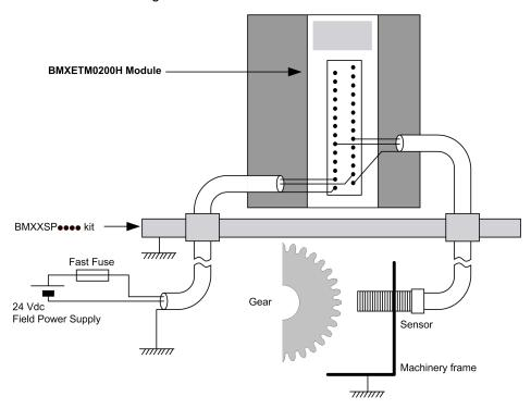
Improper fuse selection could result to damage to the module.
