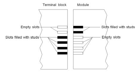
The following example depicts a coding configuration that obstructs the terminal block from fitting onto the module:
