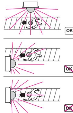
**i** The following figure shows the ranges of the detector at average temperature conditions and a mounting height of 2.20 m. The range of a movement detector can vary greatly depending on the temperature.
