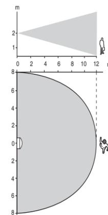
**i** Movement detectors switch on as soon as they detect a moving heat source. In order to avoid false alarms, the chosen installation site should be such that undesired heat sources cannot be detected.
