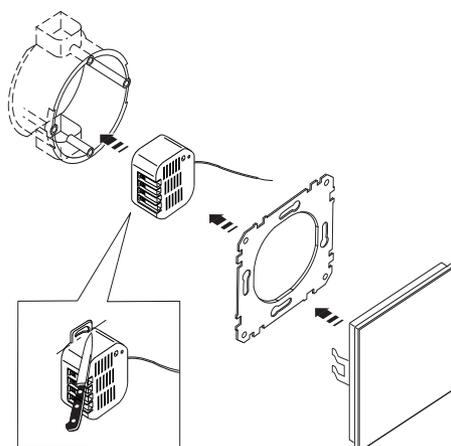
**i** Place the antenna as far as possible from metal parts (connecting cables, retaining rings, etc.) to avoid interruptions to the radio signal.
