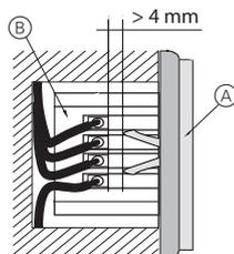
If the distance is less than 4 mm, a deeper installation box must be used.
