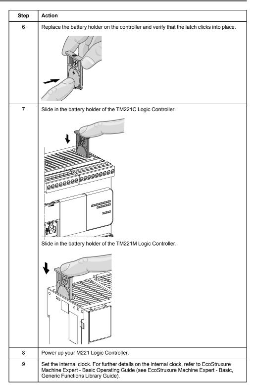
**NOTE:** Replacement of the battery in the controllers other than with the types specified in this documentation may present a risk of fire or explosion.
