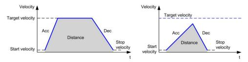
The diagram illustrates a complex profile from Continuous state:
