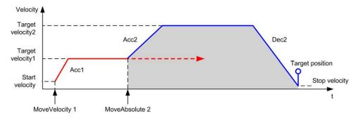
The diagram illustrates a complex profile from **Discrete** state:
