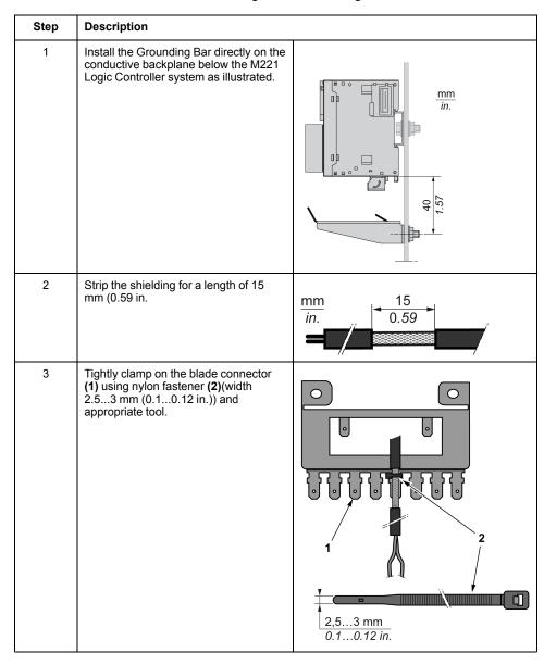
**NOTE:** Use the TM2XMTGB Grounding Bar exclusively for Functional Ground (FE) connections.
