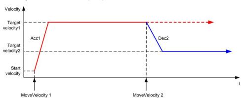
The diagram illustrates a complex profile from **Continuous** state with change of direction:
