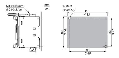
The following diagram shows the mounting hole layout for TM221C Logic Controller with 40 I/O channels:
