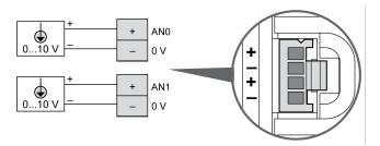
The (-) poles are connected internally.
