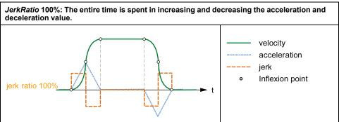
**NOTE:** The *JerkRatio* parameter value is common for acceleration and deceleration so that concave time and convex time are equal.
