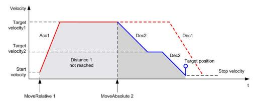
The diagram illustrates a complex profile from **Discrete** state with change of direction:
