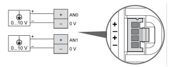
The (-) poles are connected internally.
