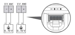
The (-) poles are connected internally.
