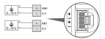
The (-) poles are connected internally.
