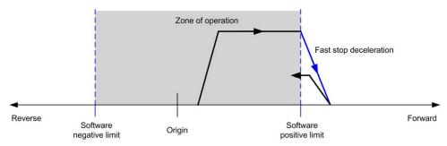
**NOTE:** In previous diagram, the axis move back in the limits is the result of the execution of *MC\_Reset\_PTO* (it is not performed automatically).
