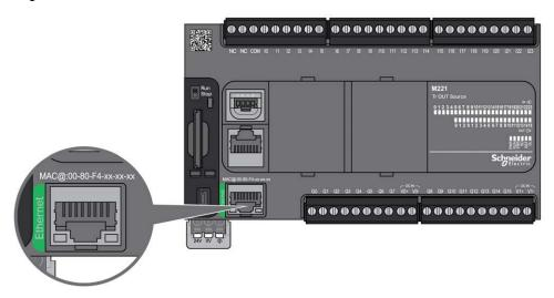
The following figure presents the location of the Ethernet port on the TM221M Logic Controller:
