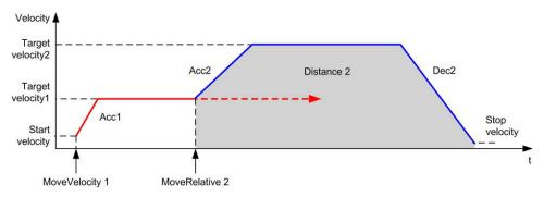
The diagram illustrates a complex profile from **Continuous** state with change of direction:
