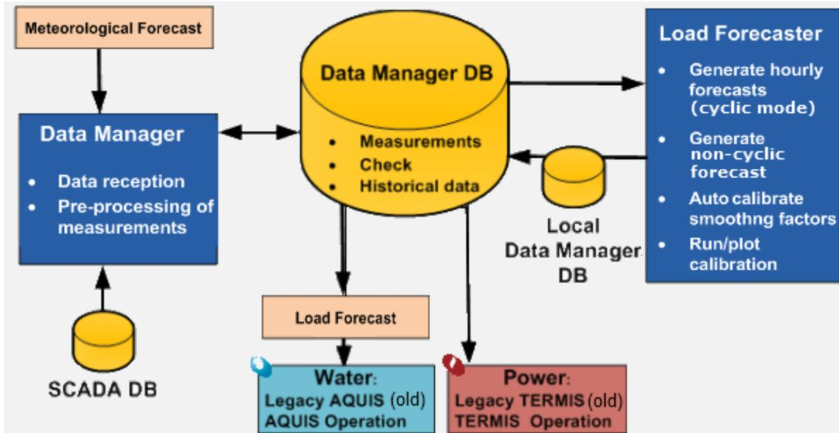
The illustration shows (to the left) how data from a SCADA database and meteorological data (for example from a national weather forecast center) are fed into a Data Manager database and processed in the Load Forecaster where after the results are sent to either legacy (old) TERMIS/AQUIS or TERMIS/AQUIS Operation.
