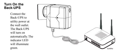
**Note:** The indicator LED will flash green if the Back-UPS is not completely charged. The Back-UPS will auto charge the battery.
