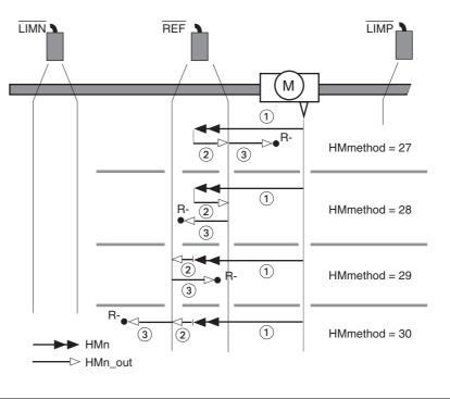
Figure 8.11 Reference movements to the reference switch
