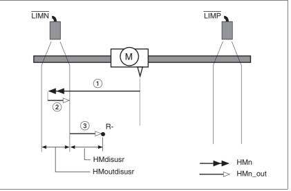
Figure 8.10 Reference movement to the negative limit switch
