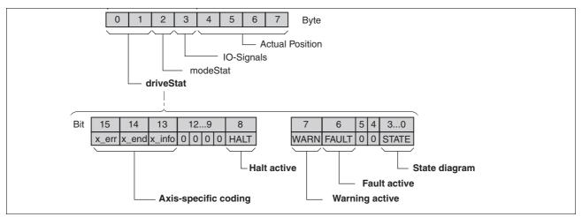
Figure 8.2 Structure of driveStat
