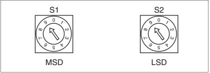
Figure 6.8 Factory settings of the rotary switches
