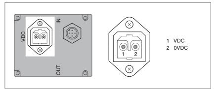
Figure 6.7 Pin assignment supply voltage
