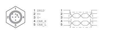
Figure 6.10 Pin assignment industrial connector
