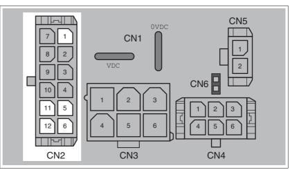
Figure 6.9 Pin assignment printed circuit board connector
