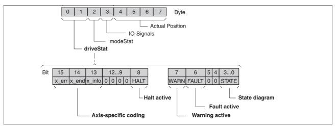
Figure 8.2 Structure of driveStat
