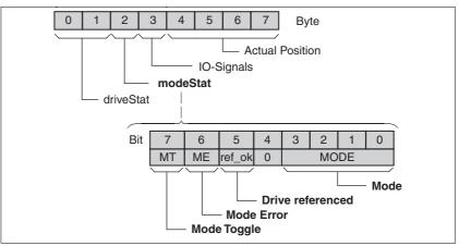
Figure 8.4 Structure of modeStat
