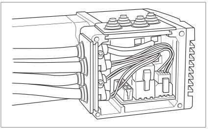
Figure 6.5 Inserting the cable entries
