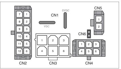
Figure 3.5 Overview of printed circuit board connectors
