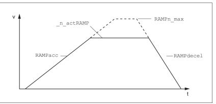
Figure 8.25 Acceleration and deceleration ramps
