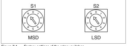
Figure 7.1 Factory settings of the rotary switches
