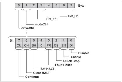
Figure 8.3 Structure of driveCtrl
