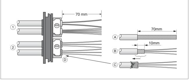
Figure 6.3 Fastening the cable in the cable entry
