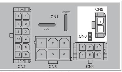
Figure 6.13 Pin assignment of safety function
