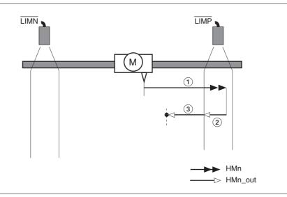
Figure 8.13 Reference movement to the positive limit switch
