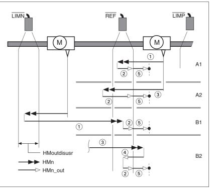
Figure 8.15 Reference movements to the reference switch
