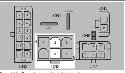
Figure 6.11 Pin assignment printed circuit board connector
