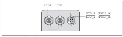
Figure 6.15 Pin assignment
