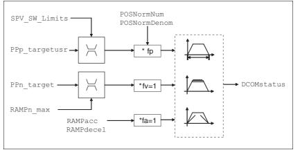
Figure 8.8 Operating mode Profile Position, effect of adjustable parameters
