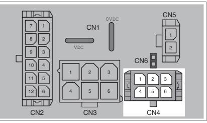
Figure 6.12 Pin assignment printed circuit board connector
