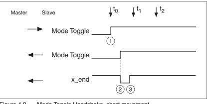
Figure 4.8Mode Toggle Handshake, short movement
