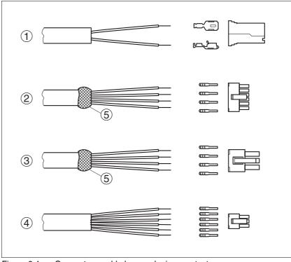
Figure 6.4 Connectors, cable lugs and crimp contacts
