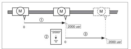
Figure 8.17 Positioning by 4000 usr units with position setting
