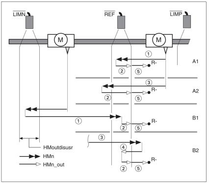
Figure 8.12 Reference movements to the reference switch
