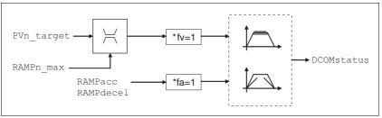
Figure 8.9 Operating mode Profile Velocity, effects of adjustable parameters
