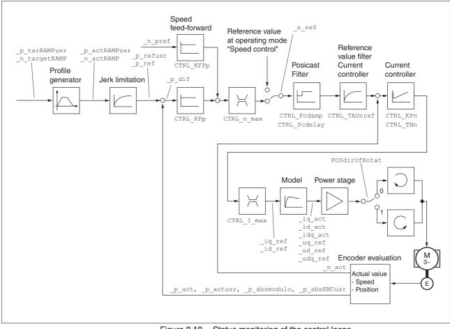
Figure 8.18 Status monitoring of the control loops
