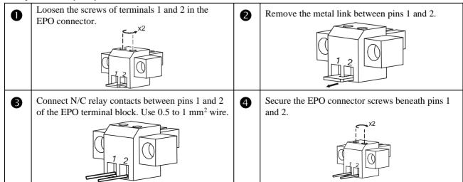
**NOTE:** If the N/C is open, the UPS will turn off and power will be removed from the load. Use Class 2 cable (CL2) to connect the Easy UPS to the EPO switch.
