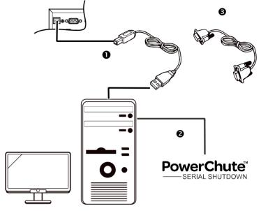
3. A built-in serial port is also available for additional communication options with serial cable. Note: RS232 and USB cannot be used at the same time
