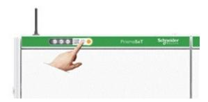
4. On the panel, **the indicator light will go from a few seconds on** solid orange to flashing green during the service activation phase. Then click **Next**.
