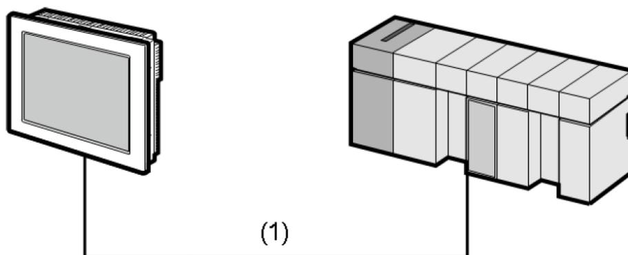
(1) Ethernet cable by Schneider Electric 490 NTC 000
