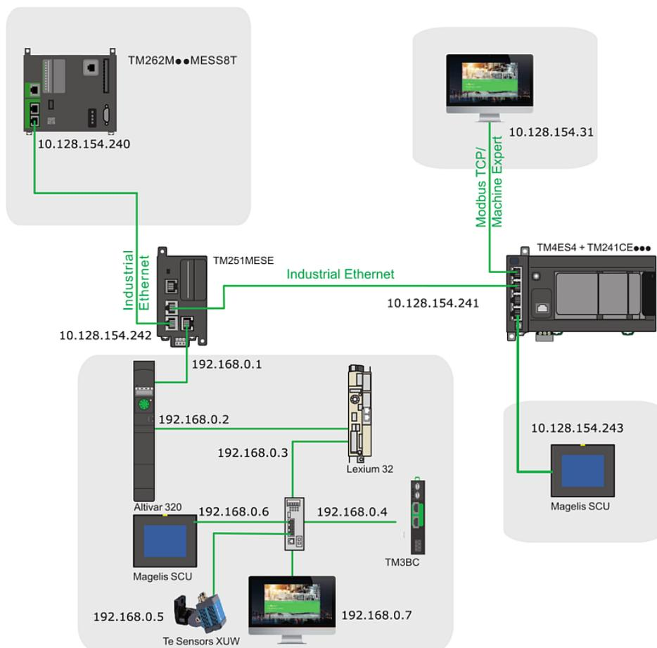
The following sections describe where a Modicon M241 Logic Controller is usually integrated.
