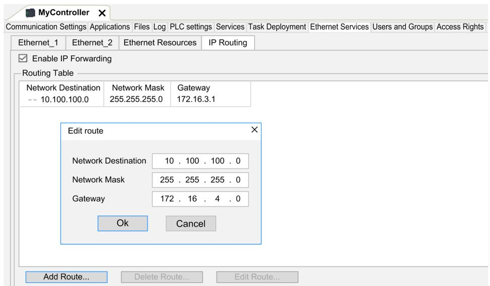
**NOTE:** On Modicon M241 Logic Controller, the **IP Forwarding** is configured in the Ethernet security parameters of the TM4ES4. On M251MESE, it is configured in the Ethernet security parameters for ETH1.
