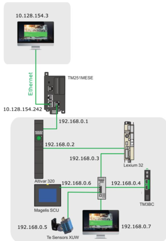
The following sections describe the typical architecture where a Modicon M251 Logic Controller is usually integrated. The architecture shows, that the Modicon M251 Logic Controller is able to communicate with different networks. One for machine control and one for device control.
