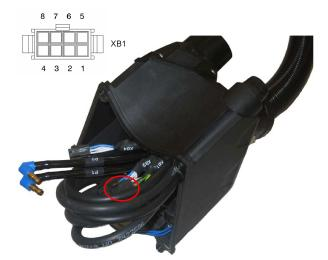
There is a one to one correspondence between the pins of the XB1 and the X1202 connectors.
