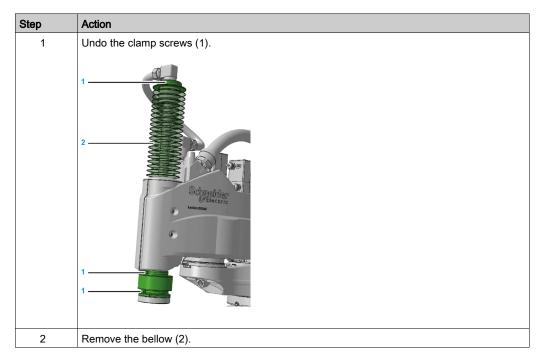
NOTE: For reassembly, use a tightening torque of 20 Nm (177 lbf-in) to tighten the clamp screws.
