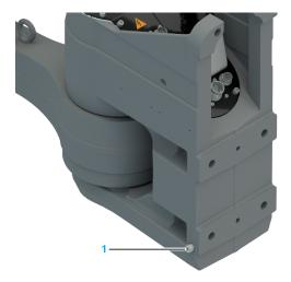
1 Ground connection at wall-mounted robot
