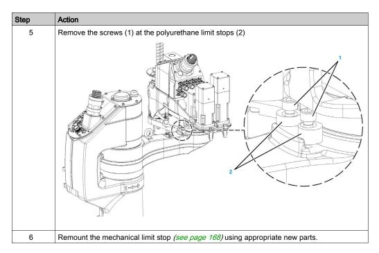
The system performance levels can only be realized when the equipment is assembled correctly with clean, degreased parts. Any failure to comply with the instructions can lead to incorrect operation of the range limiting system, with potential risks for people and equipment.
