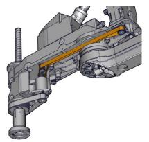
STS60/80: Position of the secondary belt on axis 4
