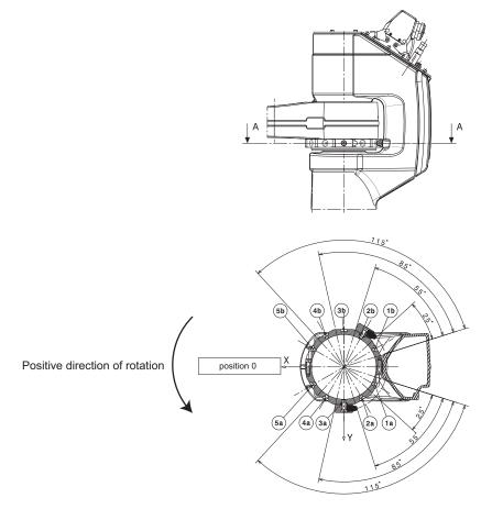
Arrays defining the ranges of the mechanical limit stop:
