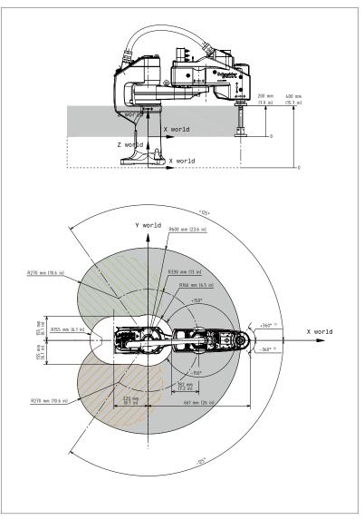
(1) 360° in either direction due to user input/output user cables - value can be adjusted if necessary. For further information, contact your local Schneider Electric service representative.
