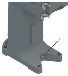
1 Ground connection at floor-mounted robot
