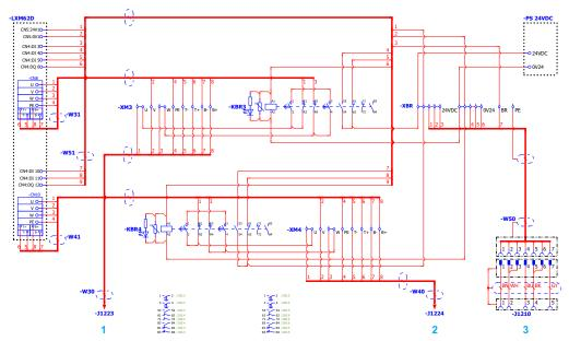
The following circuit diagram presents an example for cross-circuiting axis 3 and axis 4:
