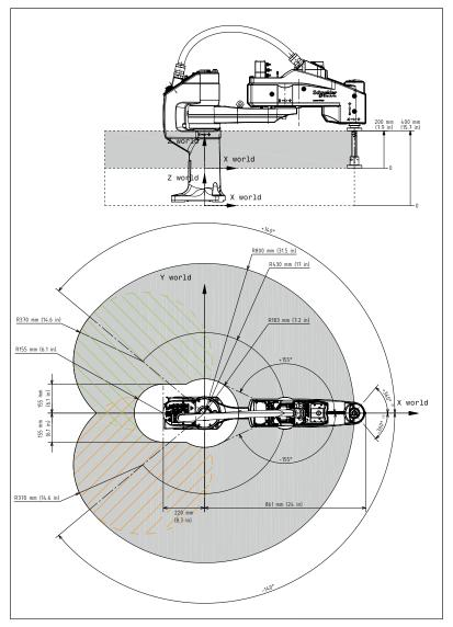
(1) 360° in either direction due to user input/output - value can be adjusted if necessary. For further information, contact your local Schneider Electric service representative.
