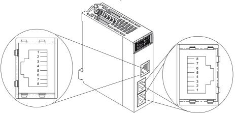
The table below shows the pin assignment for the serial port on the BMXNOM0200:
