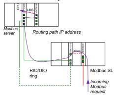
NOTE: The same path is used to route the Modbus response.
