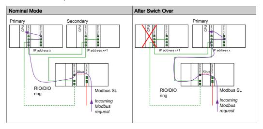
**NOTE:** The Modbus master application manages the repetition of requests in case of a message loss that could occur during a PLC switch over.
