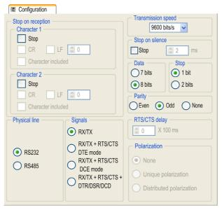
**NOTE:** In this example, the **Polarization** and **RTS/CTS delay** zones are grayed out respectively because an RS232 physical line and RX/TX signals have been chosen.
